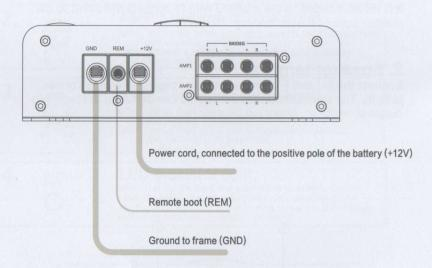
Please use 8AWG cables for power and grounding wires
