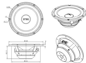
Recommended Frequency Cut: high pass up to 4.5k Hz The cuts and slopes refer to these data according to the applied power and the position of the speaker, so we can not set a reliable standard.
